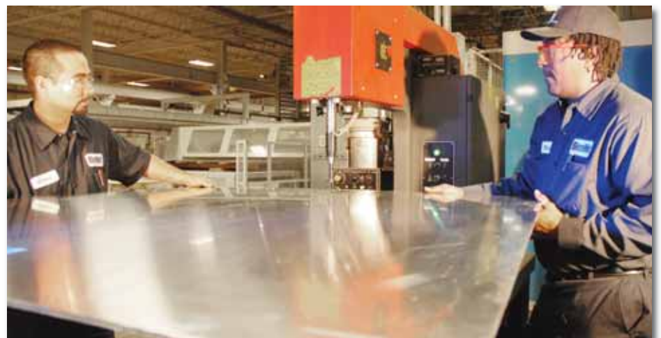
Figure 3 GenMet employees fabricated a stabilizing table to help with the handling of large parts at the hardware insertion station. Such suggestions have led to increased shop floor productivity.
