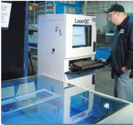
Figure 4 Several years ago GenMet employees had to wait on the company's only quality inspector to sign off on production of first pieces. Now they can use a laser scanner that sits right in the middle of the shop floor to ensure parts meet all specifications—without waiting for someone.
