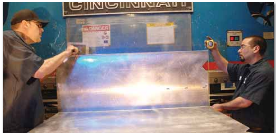
Figure 5 One of many quality inspectors can perform first-piece inspection of large parts.
